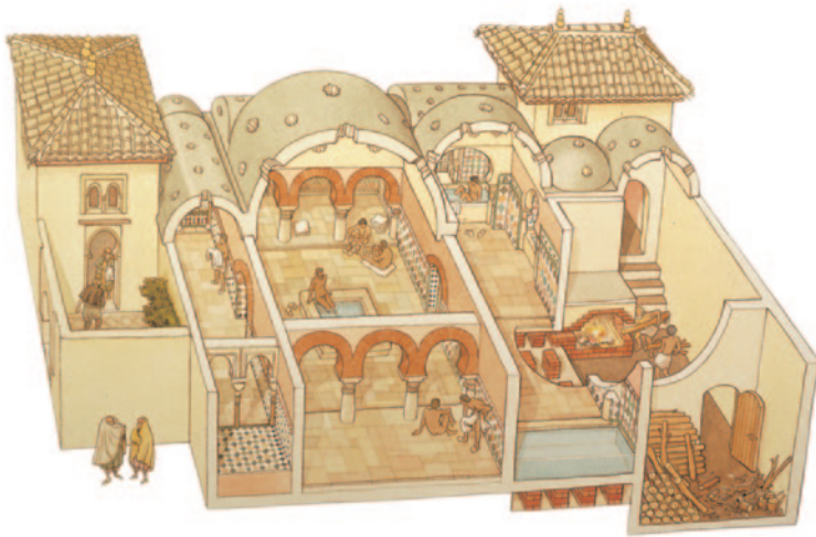
Above, typical Moorish baths, al-hammam in Arabic, origin of the name Alhama. They consist of a courtyard, a hall, a cold room, a warm room with a pool and the hot room, where the steam and hot water are produced by a boiler.
